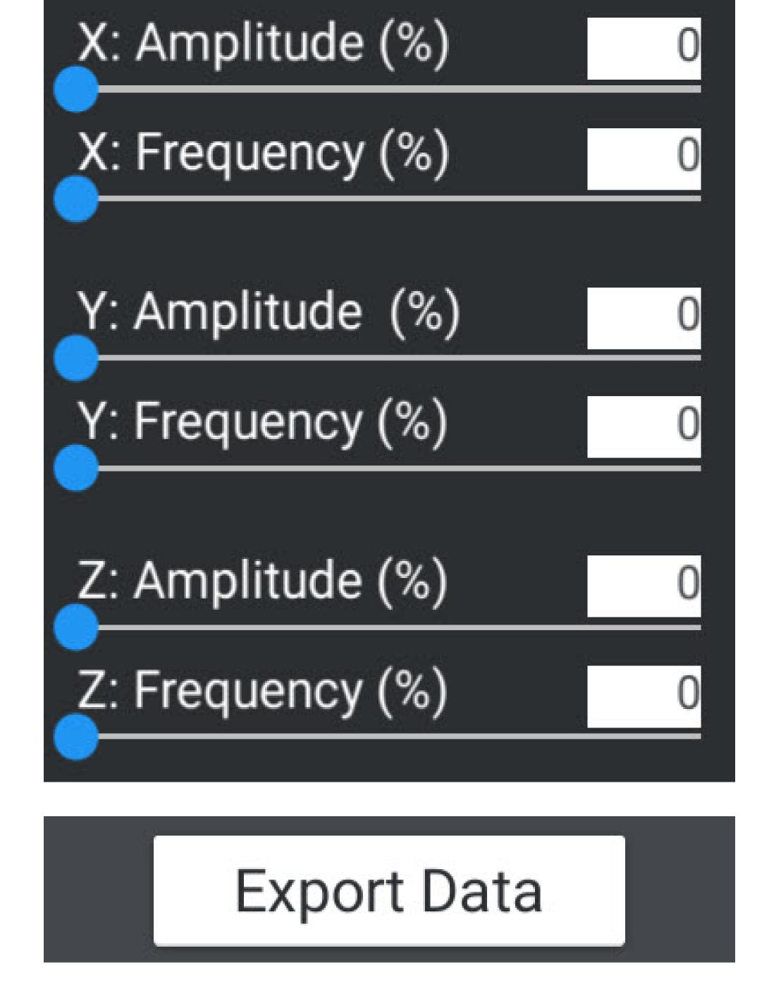
**Shake Table Controls**: Use these slider or text boxes to control the amplitude and frequency of the shake table along the x, y, and z axes.
